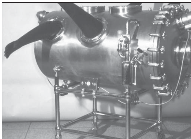
FIG. 1. The steam sterilized isolator system.
